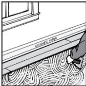
Lay the first row of starter boards along the chalk line/straight edge. Starting from the left corner, secure the boards into position with tongue-side facing the wall.
