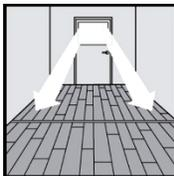
Boards shall run lengthwise against the longest wall. When possible try to run floor boards parallel to incoming sunlight or main light source.
